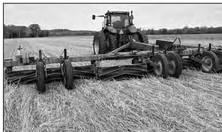
ROLLER CRIMPING: Roller crimping cover crop at Big River Grain and Cattle. Roller crimping flattens and terminates the cereal rye, creating a mulch that protects the soil and suppresses weeds. (Photos courtesy of Daniel Bonacker)
